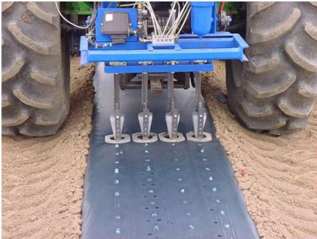
First design of a Dibbling machine that can be reconfigured rapidly for different planting configurations
